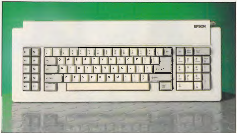
The layout is good but there are no LEDs to show when keys are engaged
